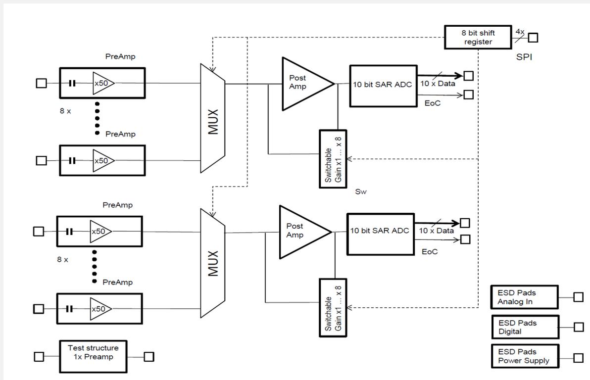
Figure 2: Block Diagram ECoG3 Chip
