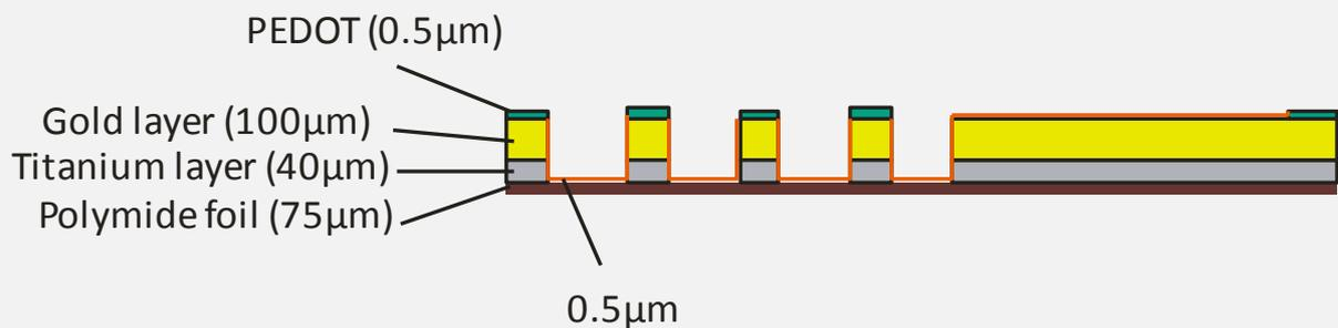
*Fig. 2 Cross section of flexible electrode using a polymide foil as a substrate.*
