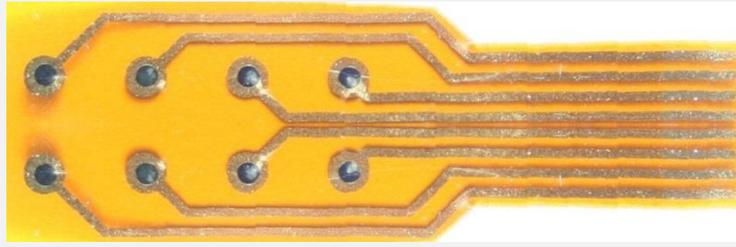
Fig. 3 Metallization level and PEDOT deposition (Black circles) for electrodes with reduced impedance
